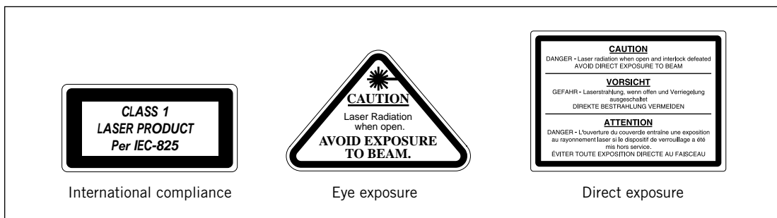
Figure 2-8. Laser-light warning labels.
