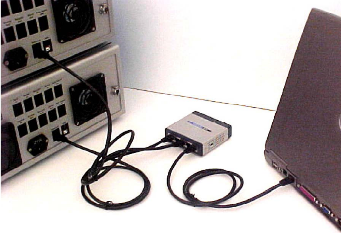
Figure D-17: Connecting multiple instruments to a computer not on the LAN using an Ethernet switch.
