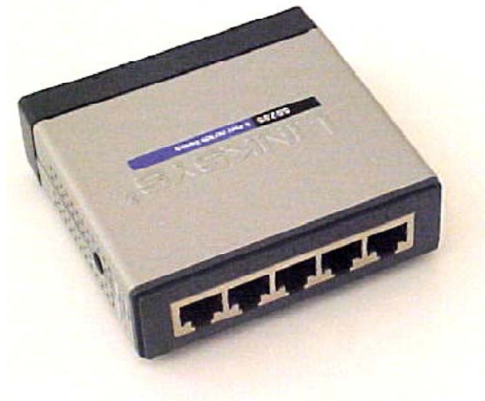
Figure D-7: Five-port Ethernet switch.
