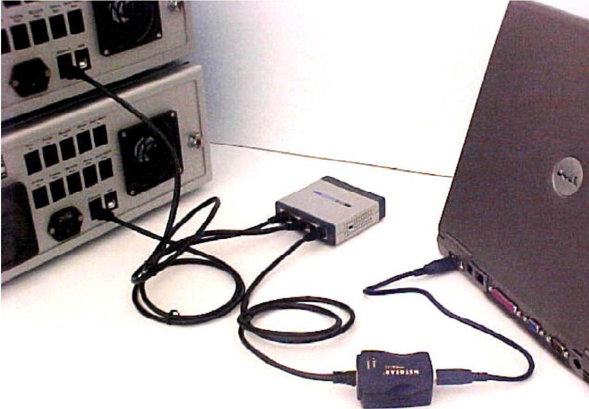
Figure D-14: Connecting two or more instruments to USB using an Ethernet switch and Ethernet to USB adapter.
