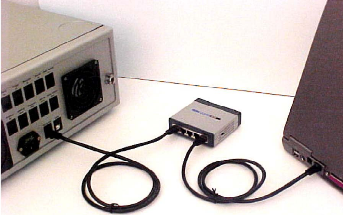
Figure D-16: Connecting one instrument to the computer using an Ethernet switch.
