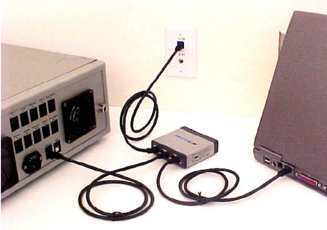
Figure D-9: One instrument and a computer can both be connected to the LAN using an Ethernet switch.
