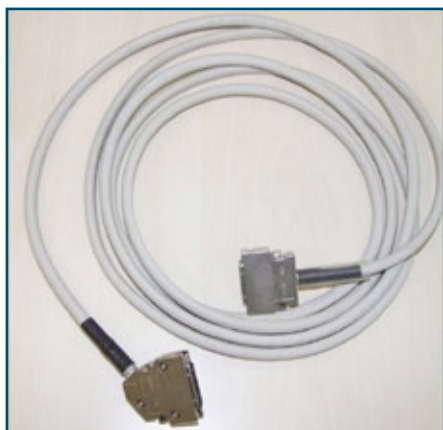
Figure 5: PCI controller card to camera cable
