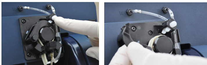
Figure 6.3 Release Pump Tubing Pressure Plate
