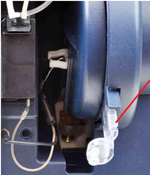
Figure 6.14 Replacing the Safety Sample Port
