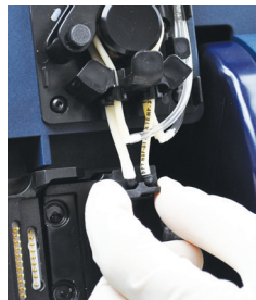
Figure 6.4 Disconnect Pump Manifold
