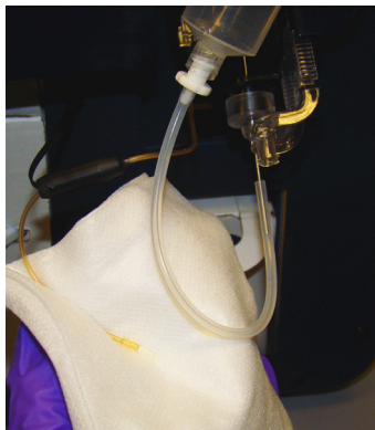
Figure 7.5 Flushing the S-Line
