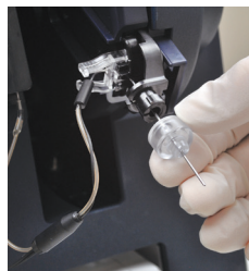
Figure 6.7 Removing Capillary Adapter
