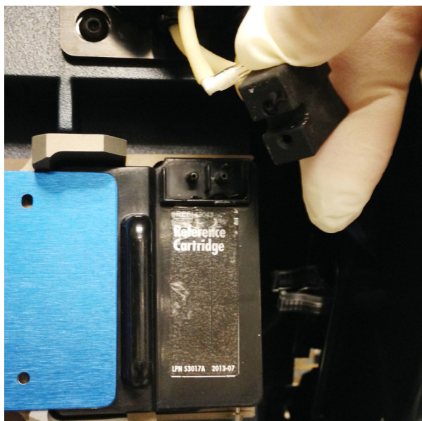
Figure 6.5 Connect Tubing Connector to Reference Sensor
